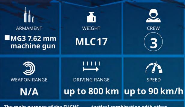
The main purpose of the FUCHS APC (armoured personnel carrier) "HUMMEL 05/06" is to jam enemy radio communication systems by using electronic countermeasures in different frequency ranges. The HUMMEL 05/06 works in tactical combination with other electronic countermeasure systems and may be assigned to a brigade or division. In a national and collective defence scenario, the HUMMEL 05/06 will be deployed 10 km behind the forward edge of battle area (FEBA).
