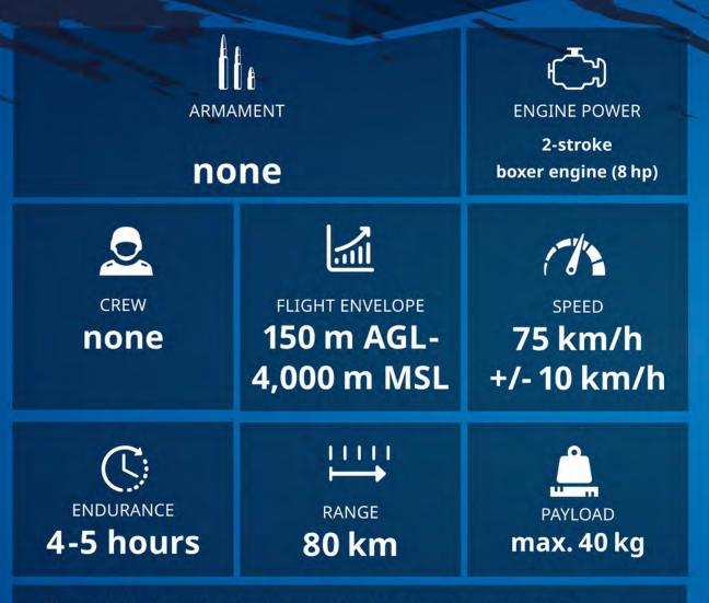
The LUNA UAS is a lightweight, during day and night. easy-to-operate Real-time aerial easy-to-operate reconnaissance system for real-time, close-range aerial reconnaissance and surveillance using video, infrared film and still images
