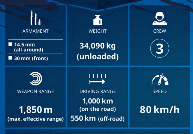
The Boxer GNGP is a multi-purpose vehicle that can be used as an infantry, engineer and medical vehicle. Different mission modules can be attached to the drive module within one hour. The infantry module we use provides seating for six dismounts and offers protection against several AT weapons and up to 10 kg AT mines. It is armed with an <u>M151</u> Protector RCWS (.50 cal.).
